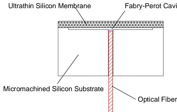
**Figure 7 -- Davidson's MEMS Fiber-Optic Pressure Sensor**
