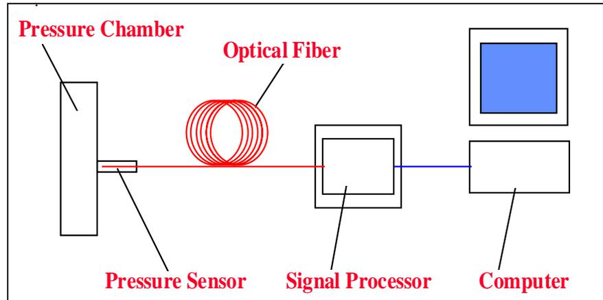
*Figure 2 – Fiber Optic Sensing System*
