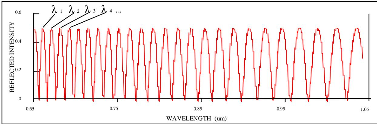
Figure 4 – Intensity of Conditioned Light reflected from the Fabry-Perot Interferometer
