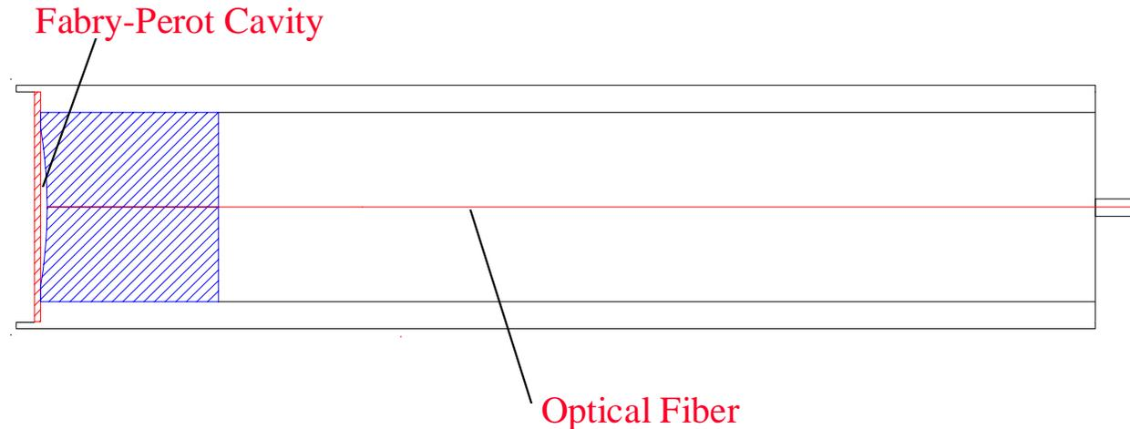
**Figure 6 – Fabry-Perot Fiber Optic Sensor**
