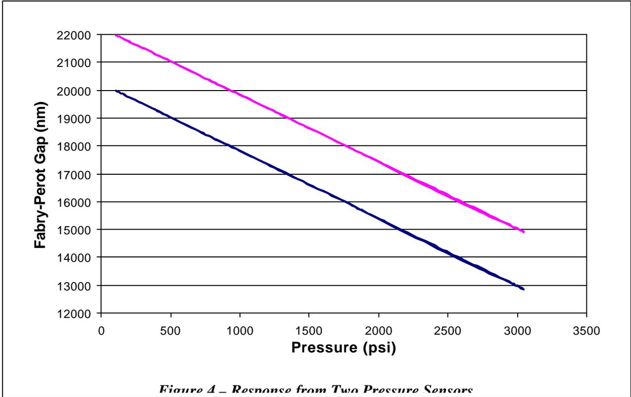
*Figure 4 – Resonance from Two Pressure Sensors*
