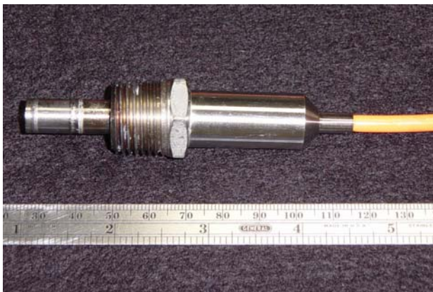
Fig.1 Photo of fiber optic pressure transducer assembly and cable.
